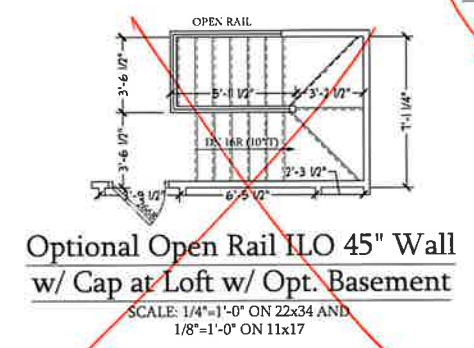
Optional Open Rail ILO 45" Wall w/ Cap at Loft SCALE: 1/4"=1'-0" ON 22x34 AND 1/8"=1'-0" ON 11x17
