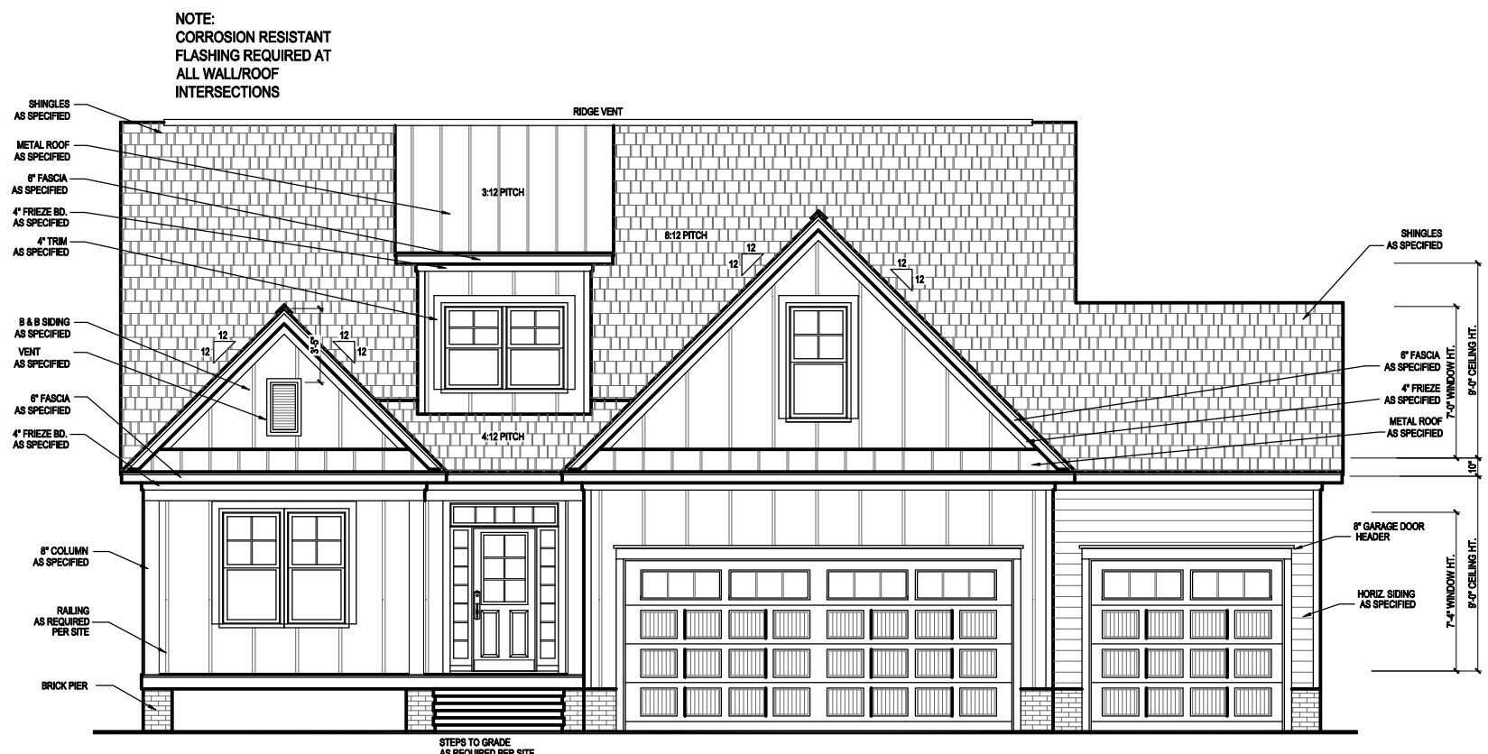
FRONT ELEVATION - 3 CAR GARAGE SCALE: 1/8"=1'-0" (11"x17" SHEET SIZE) SCALE: 1/4"=1'-0" (24"x36" SHEET SIZE)
