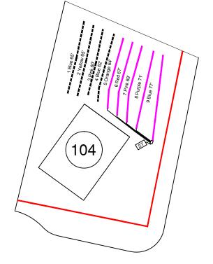
System: Gravity to D-Box Lines: 5-9, (5 x 60' x 3') Accepted Status System 0.3 Soil LTAR 24" Trench Bottom
