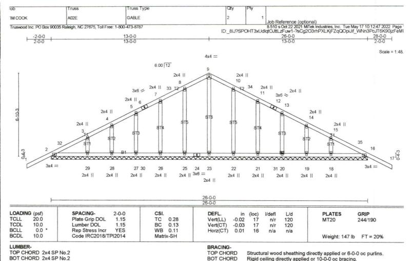
MiTek recommends that Stabilizers and required cross bracing be installed during truss erection, in accordance with Stabilizer
