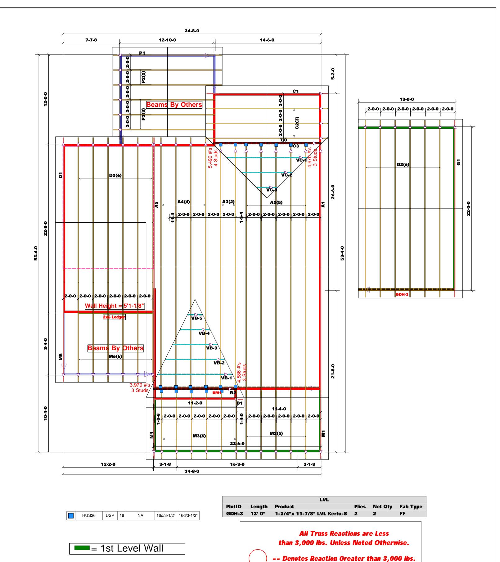
**Truss Placement Plan**
