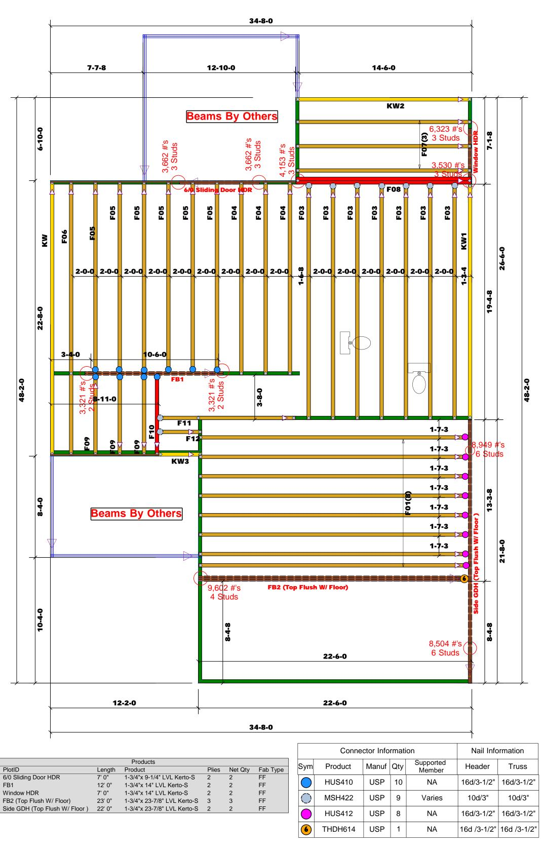
Truss Placement Plan
