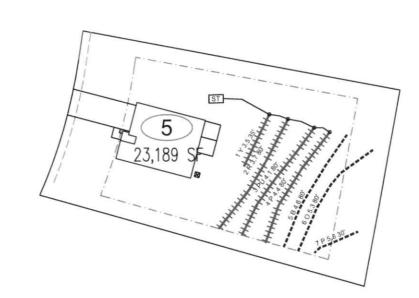
\*Keep tanks and drain lines 10' from property lines.
