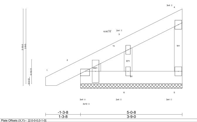
LOADING (psf) SPACING-2-0-0 CSI. DEFL. I/defI L/d **PLATES GRIP** (loc) TCLL 20.0 Plate Grip DOL 1.15 TC 0.03 Vert(LL) 0.00 n/r 120 MT20 244/190 Lumber DOL ВС Vert(CT) **TCDL** 10.0 1.15 0.01 -0.00 n/r 120 **BCLL** 0.0 Rep Stress Incr YES WB 0.03 Horz(CT) 0.00 n/a n/a **BCDL** 10.0 Code IRC2015/TPI2014 Matrix-P Weight: 27 lb FT = 20%
