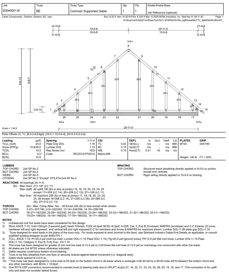
12) This truss is designed in accordance with the 2015 International Residential Code sections R502.11.1 and R802.10.2 and referenced standard ANSI/TPI 1.
