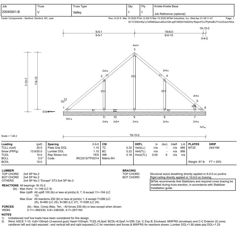
3) TCLL: ASCE 7-10; Pr=20.0 psf (roof live load: Lumber DOL=1.15 Plate DOL=1.15); Pg=20.0 psf (ground snow); Pf=13.9 psf (flat roof snow: Lumber DOL=1.15 Plate
