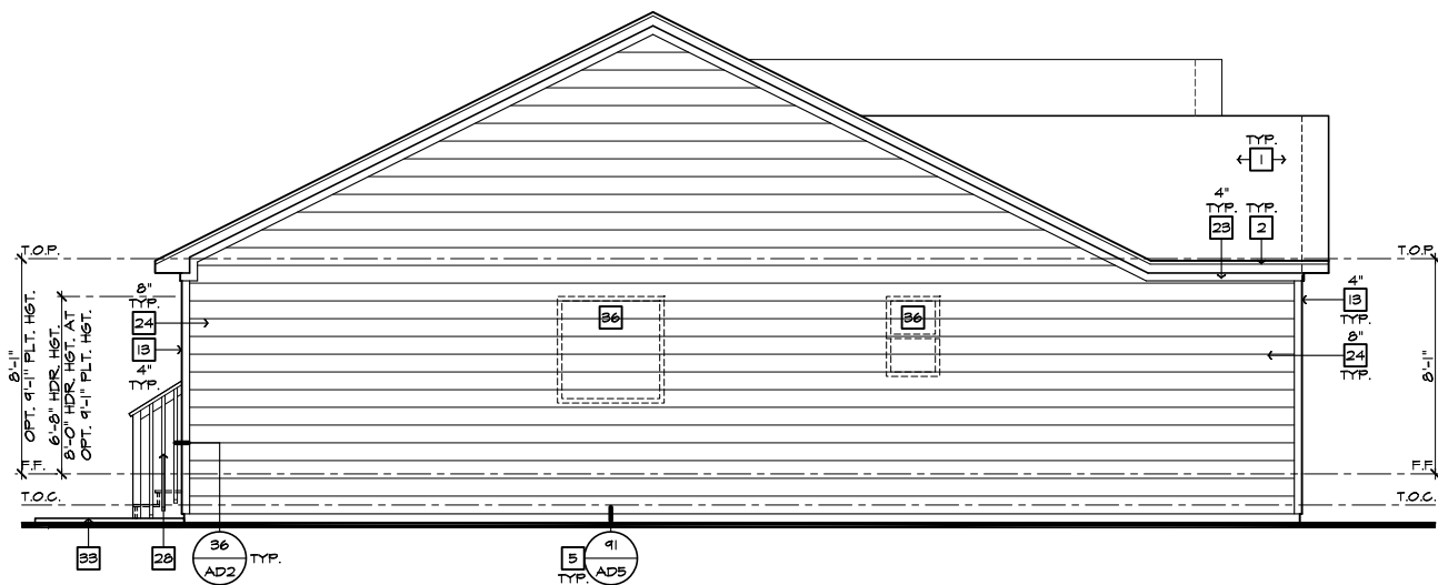
LEFT ELEVATION 'A' AT CRAWL SPACE
