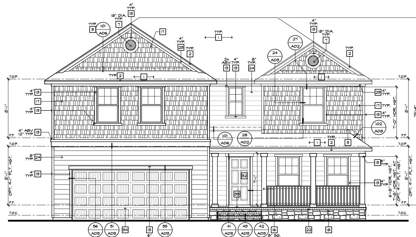
FRONT ELEVATION 'D' W/ CRAWL SPACE
