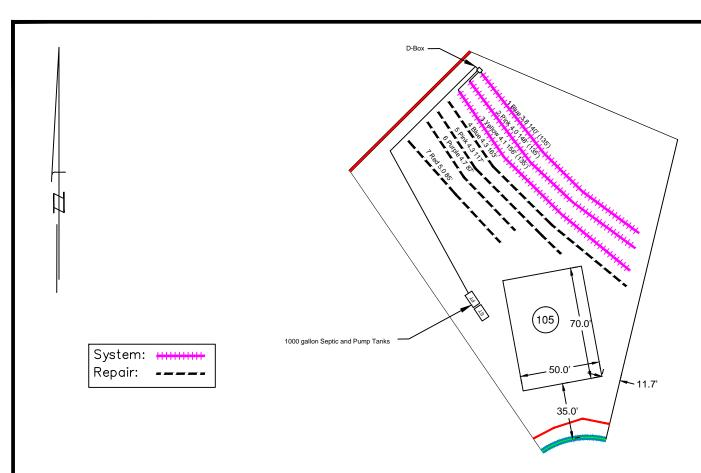
\*Keep tanks and drain lines 10' from property lines.
