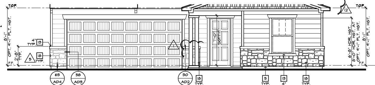
PARTIAL FRONT ELEVATION 'B' W/ STONE OPTION
