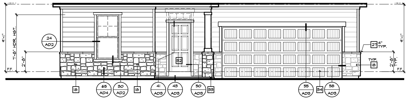
PARTIAL FRONT ELEVATION 'D' AT OPTIONAL 9'-1" PLT. HGT. W/ STONE OPT. SCALE 1/4"=1'-0" (22'x34") - 1/8"=1'-0" (11'x17")
