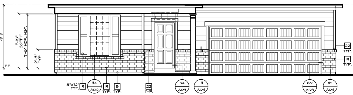
PARTIAL FRONT ELEVATION 'A' AT OPTIONAL 9'-1" PLT. HGT. W/ STONE OPT. SCALE 1/4"=1'-0" (22"X34") - 1/8"=1'-0" (11"X17")
