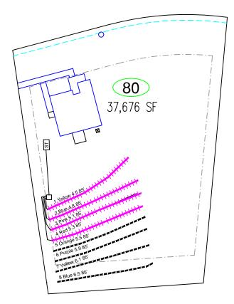
System: Gravity to D-Box Lines: 1-4, (4x85'x3') Accepted Status System 0.35 Soil LTAR
