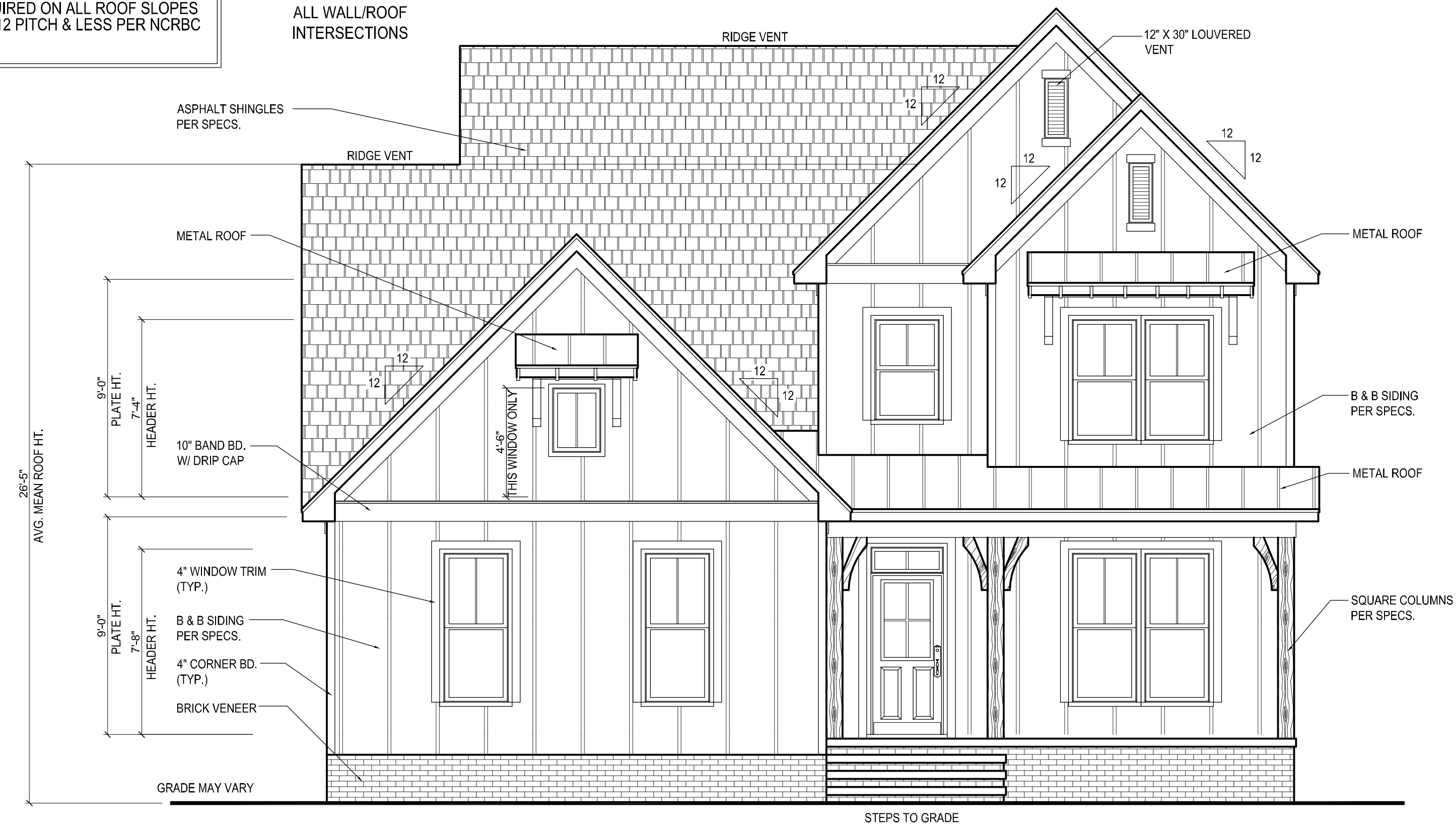
1 FRONT ELEVATION SCALE: 1/4" = 1'-0"
