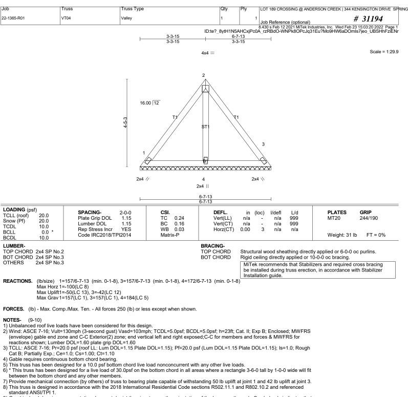
9) Graphical web bracing representation does not depict the size, type or the orientation of the brace on the web. Symbol only indicates that the member must be braced.
