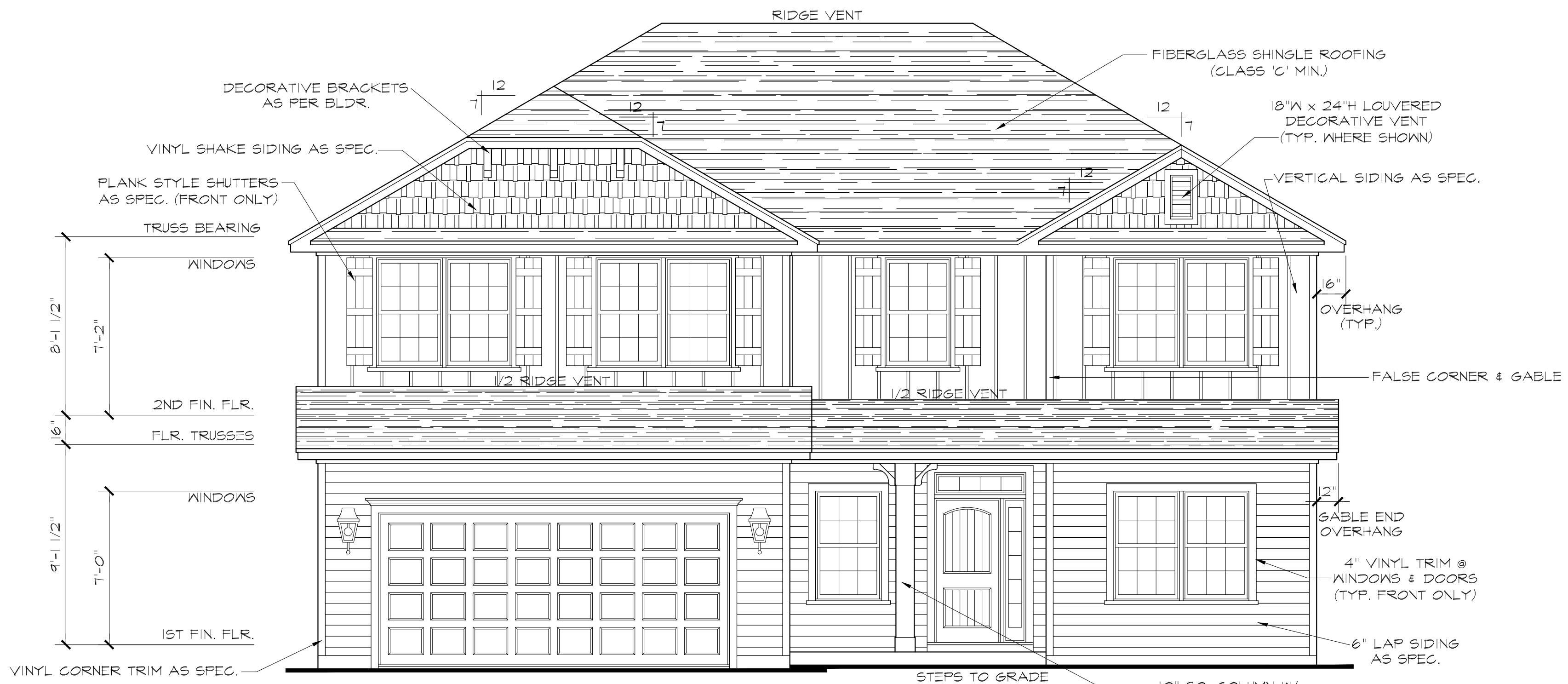
FRONT ELEVATION B SCALE: 1/4"=1'-0" NOTE - SLOPE ALL GRADES AWAY FROM HOUSE FOR POSITIVE DRAINAGE
