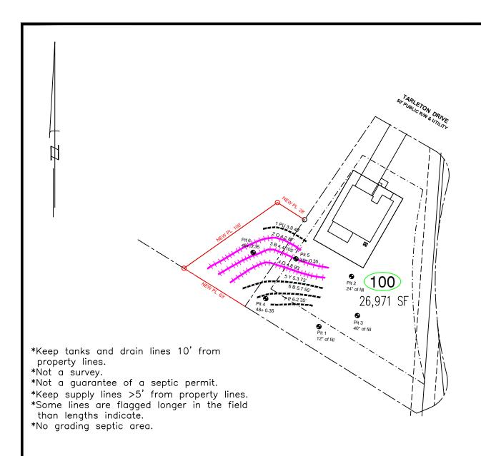
System: Gravity to Serial Dist. Lines: 2-4 (282')
