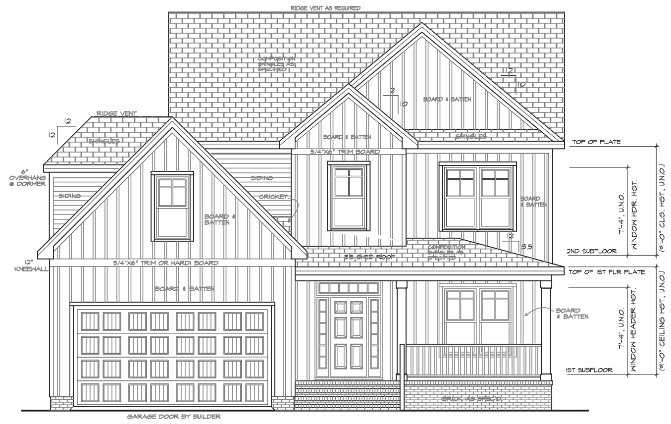
FRONT ELEVATION SCALE 1/4" = 1'0" OR SCALE 1/8" = 1'0" THIS PLAN DESIGNED UNDER NORTH CAROLINA RESIDENTIAL CODE 2018 EDITION (2015 IRC) NC (2018 NRC) : WIND : 115 - 120 MPH
