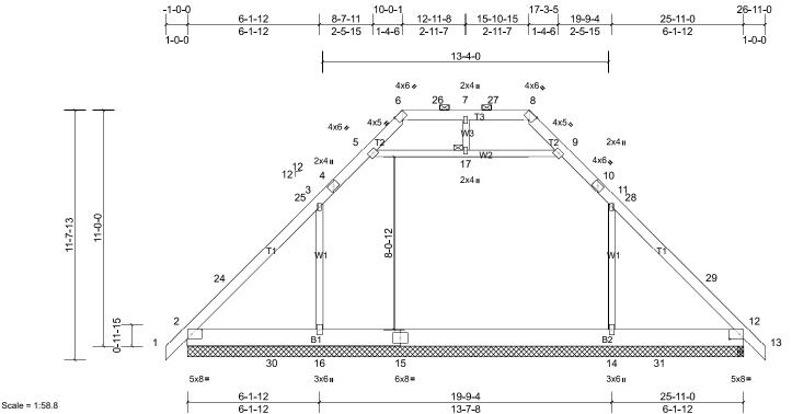
Plate Offsets (X, Y): [2:0-2-9,Edge], [6:0-2-2,Edge], [8:0-2-2,Edge], [12:0-2-9,Edge]
