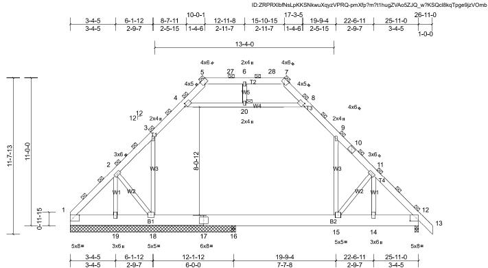
Plate Offsets (X, Y): [1:0-2-9,Edge], [4:0-1-13,0-2-0], [5:0-2-2,Edge], [7:0-2-2,Edge], [8:0-1-13,0-2-0], [12:0-2-9,Edge]
