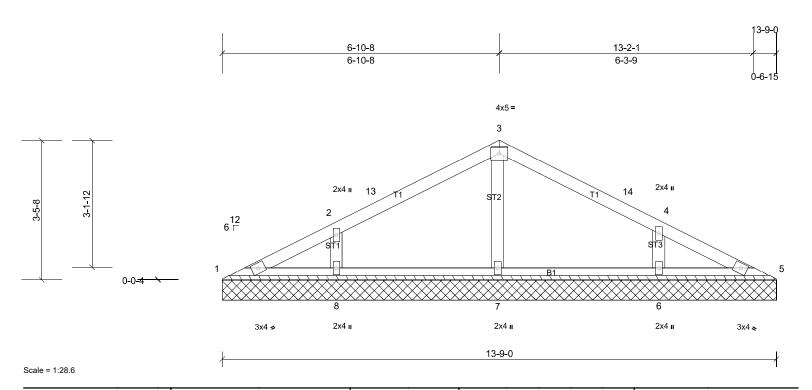
Loading (psf) **Spacing** 2-0-0 CSI **DEFL** (loc) I/defl L/d **PLATES GRIP** TCLL (roof) 20.0 Plate Grip DOL 1.15 TC 0.15 Vert(LL) n/a 999 MT20 244/190 n/a 1.15 BC **TCDL** 10.0 Lumber DOL 0.06 Vert(TL) 999 n/a n/a **BCLL** 0.0 Rep Stress Incr YES WB 0.06 Horiz(TL) 0.00 5 n/a n/a **BCDL** IRC2015/TPI2014 10.0 Code Matrix-MS Weight: 48 lb FT = 20%
