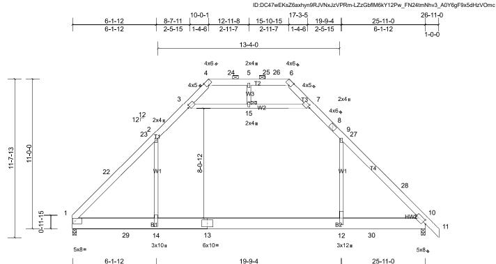
Plate Offsets (X, Y): [1:0-2-9,Edge], [3:0-1-13,0-2-0], [4:0-2-2,Edge], [6:0-2-2,Edge], [7:0-1-13,0-2-0], [10:0-2-8,0-2-8], [14:0-7-4,0-1-8]
