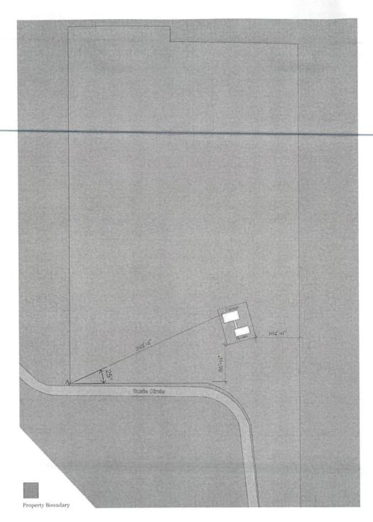
Proposed ~60'x60' building site is located 393'2" at a 25 degree angle from point A, referencing Susie Circle = 0 degrees
