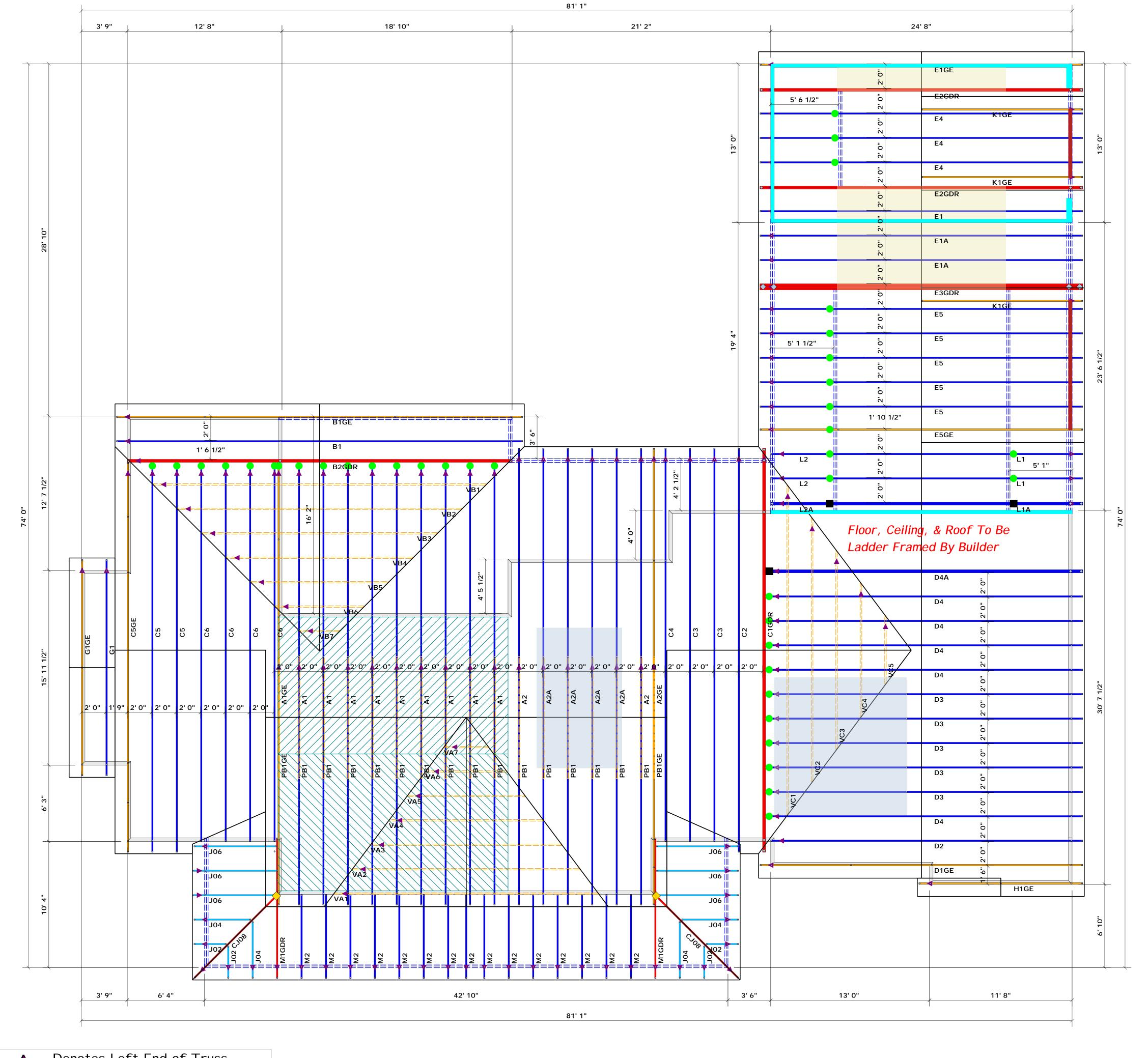
Hatch Legend 1st Floor Walls Dropped 1' 2nd Floor Bearing Walls @ 9' 1-1/2" Bonus Room, 40 lbs. Live Load Tray Ceiling Cathedral Ceiling
