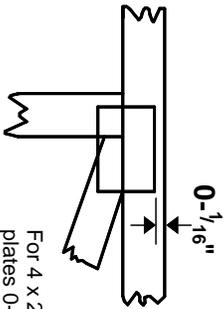
For 4 x 2 orientation, locate plates 0-  $\frac{1}{16}$ " from outside edge of truss.
