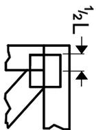
Center plate on joint unless x, y offsets are indicated. Dimensions are in ft-in-sixteenths. Apply plates to both sides of truss and fully embed teeth.
