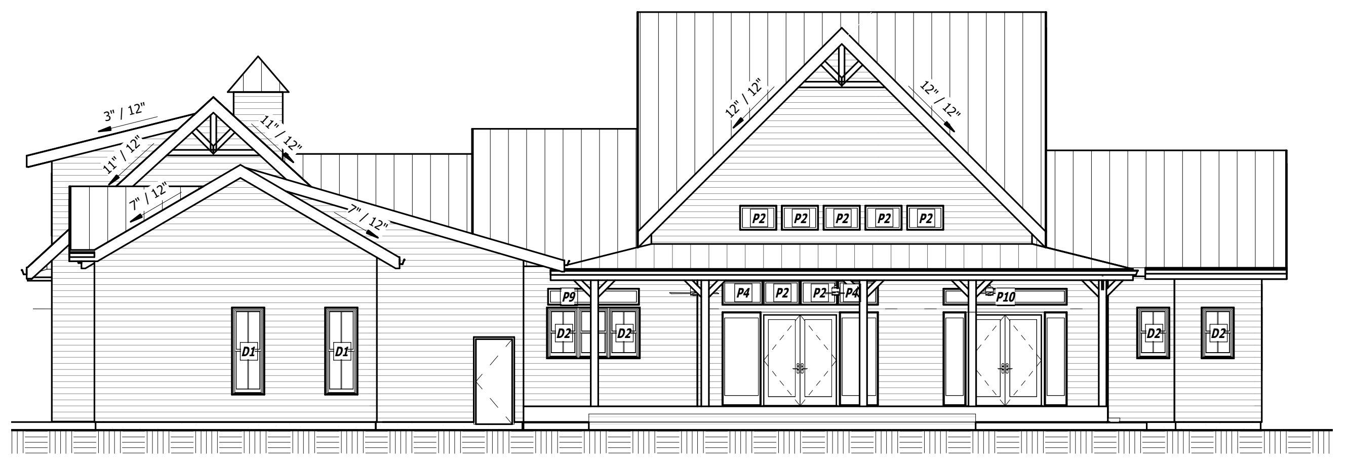
3 REAR / EAST ELEVATION SCALE: 1/8" = 1'-0"
