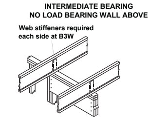
B3 B3W Blocking panels may be required with shear walls above or below (See detail B1)
