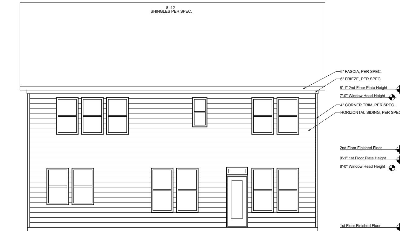
WILLOW REAR ELEVATION SCALE: 1/8"=1'-0" (11"x17" SHEET SIZE) SCALE: 1/4"=1'-0" (22"x34" SHEET SIZE)
