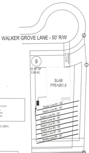
This drawing represents a preliminary septic plan made prior to final construction activities. A revised plan may need to be reworked at time of permitting.
