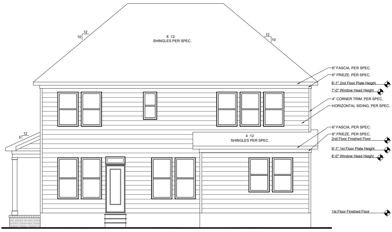
OPT. GUEST SUITE REAR ELEVATION SCALE: 1/8"=1'-0" (11"X17" SHEET SIZE) SCALE: 1/4"=1'-0" (22"X34" SHEET SIZE)
