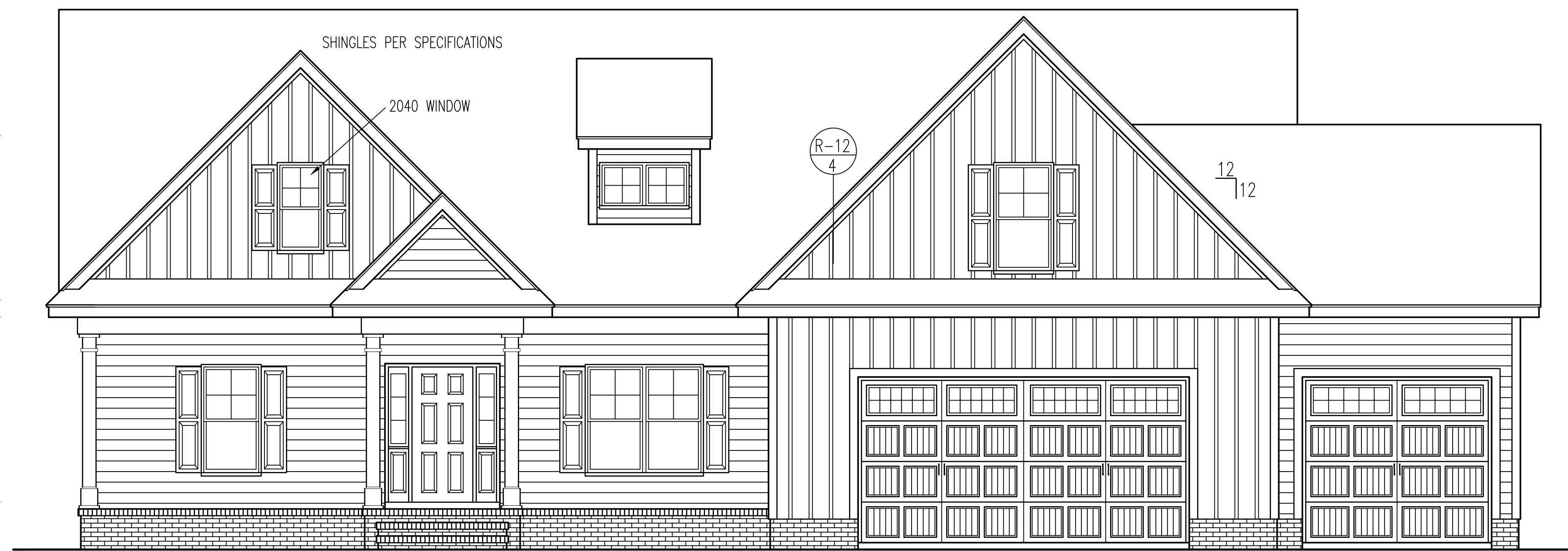
FRONT ELEVATION SCALE: 1/4" = 1'-0"
