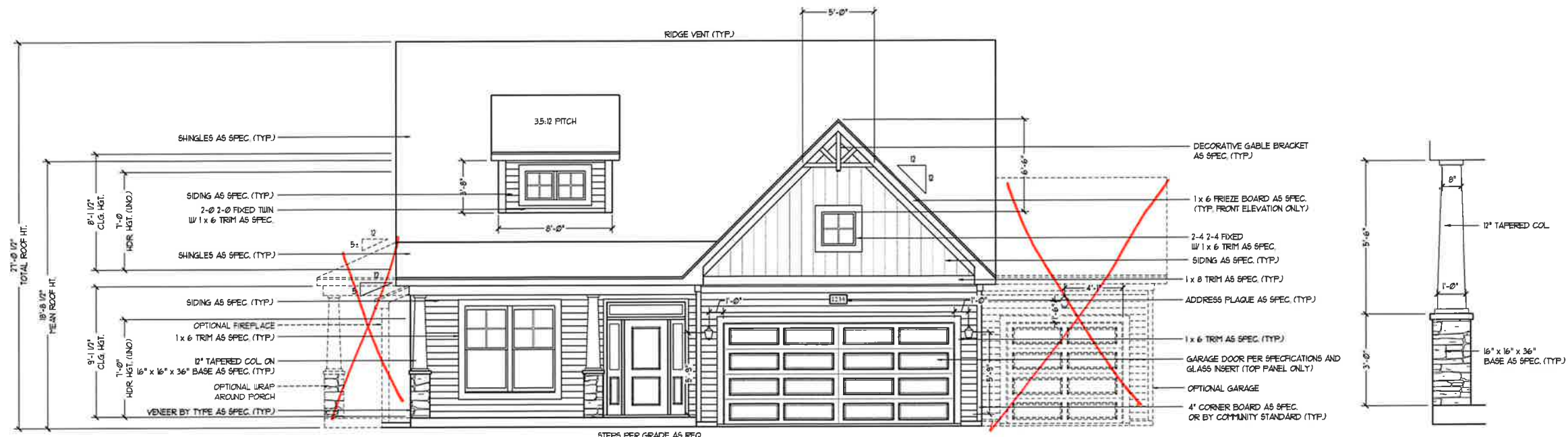
FRONT ELEVATION-B-1 SCALE: 1/4" = 1'-0"
