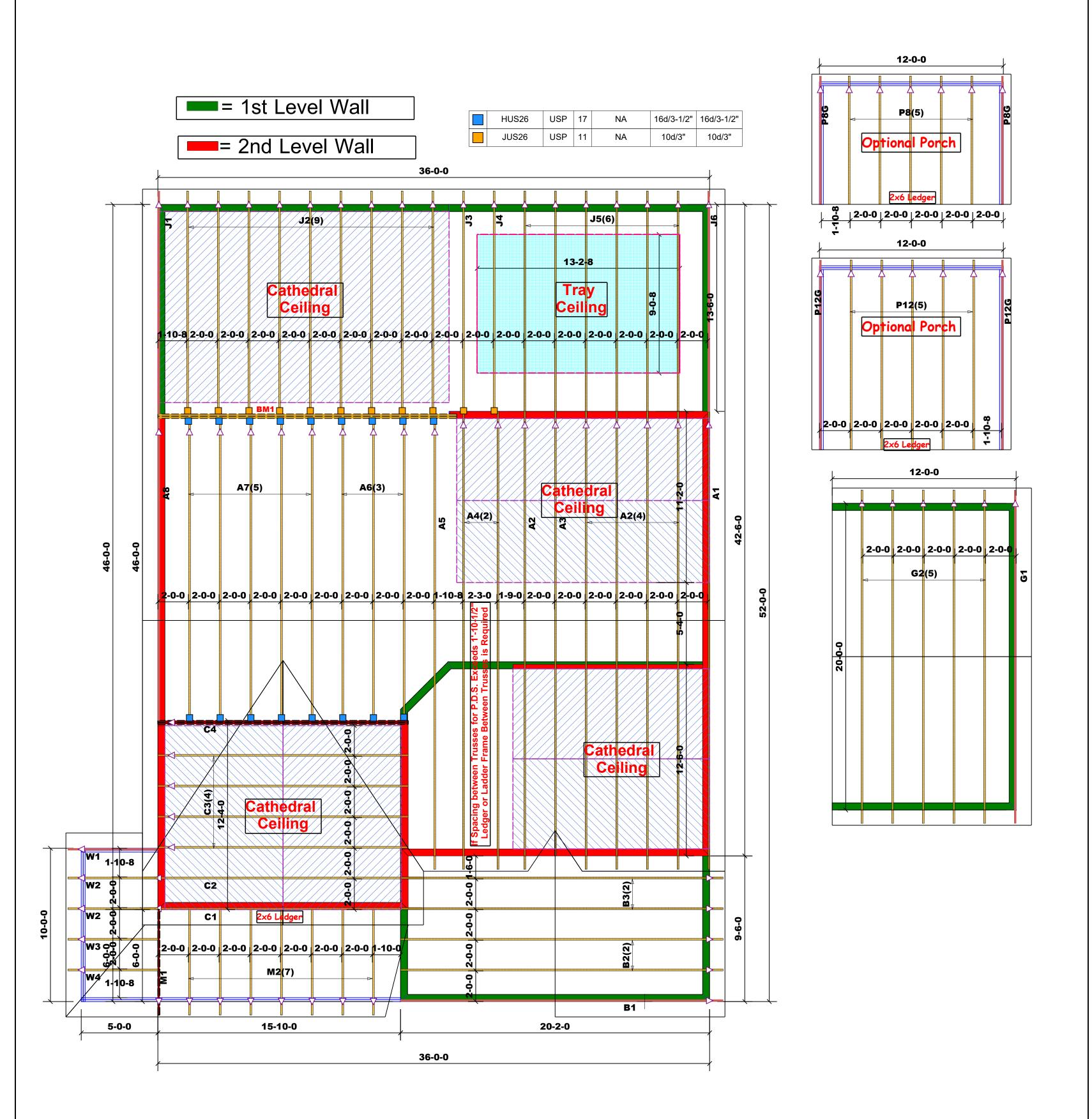
= Indicates Left End of Truss (Reference Engineered Truss Drawing) Do NOT Erect Truss Backwards
