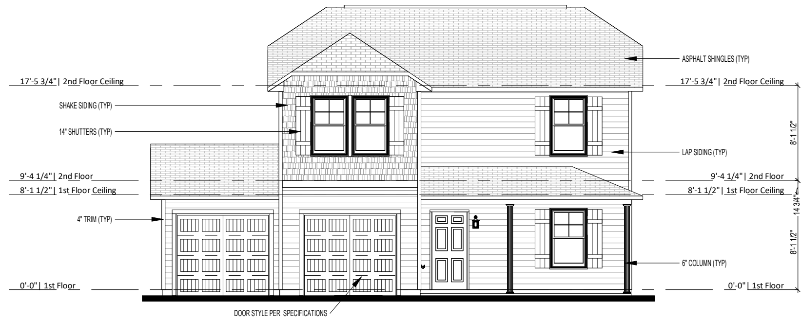
1 Front Elevation - Elev B - 2 Car Garage 1/8" = 1'-0"
