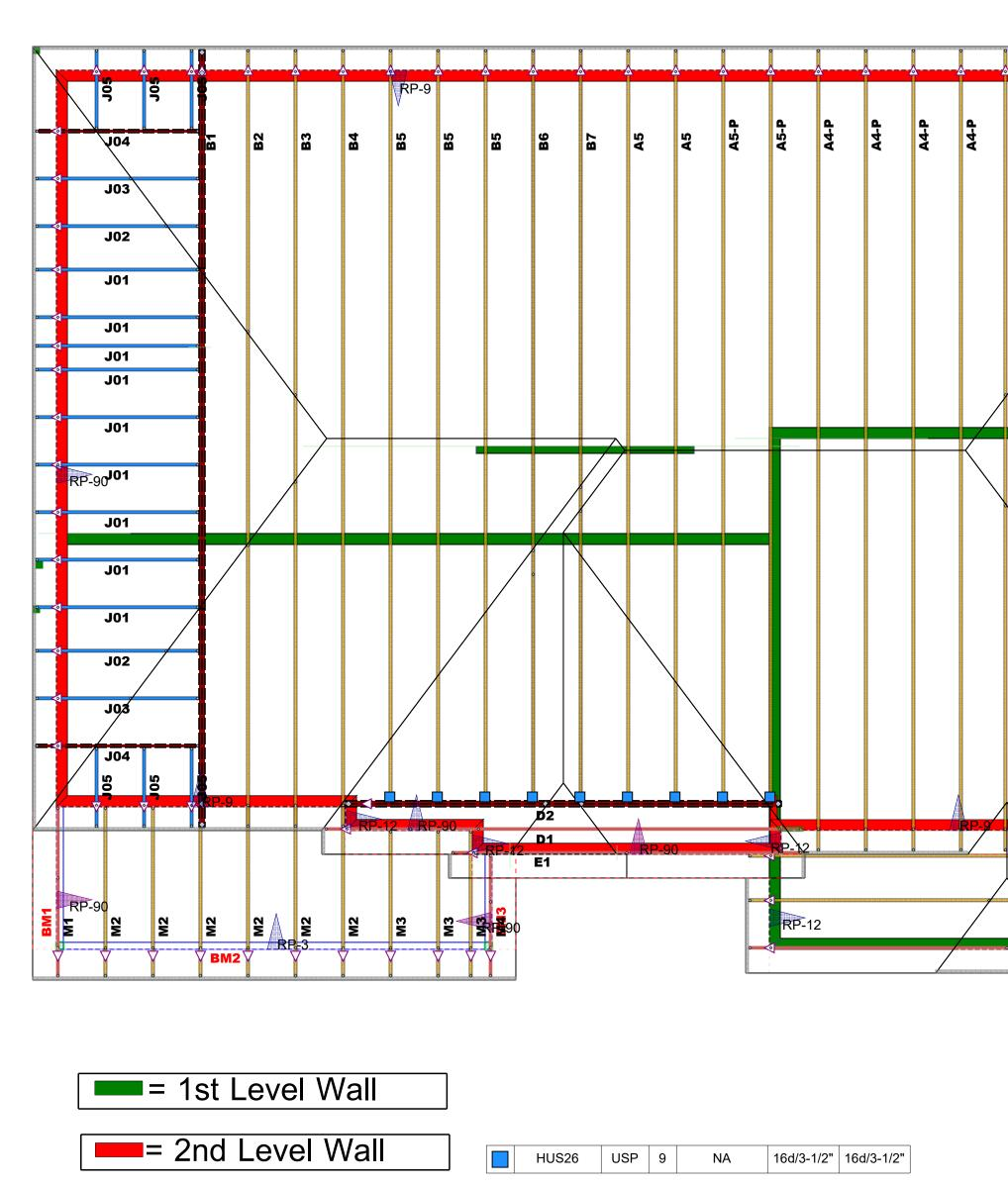
Truss Placement Plan SCALE: NTS
