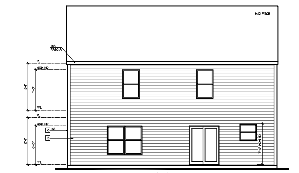
Rear Elevation 'B' SCALE: 1/8"=1'-0" AT 22'X34" LAYOUT 1/8"=1'-0" AT 11'X11" LAYOUT
