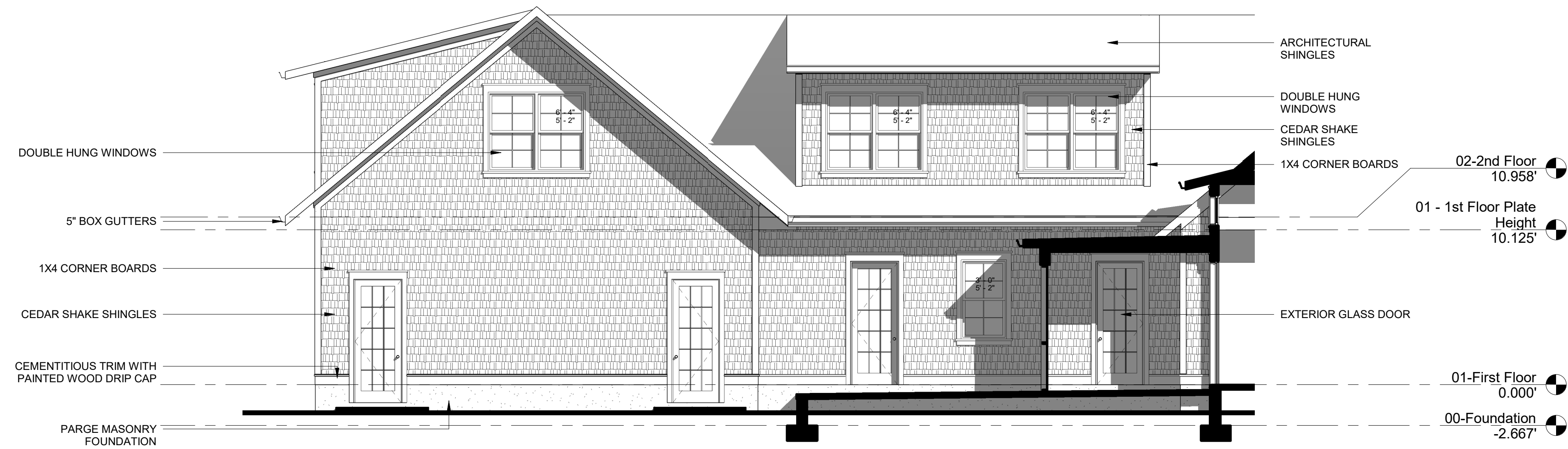
2 | Garage Rear Elevation 3/16" = 1'-0"
