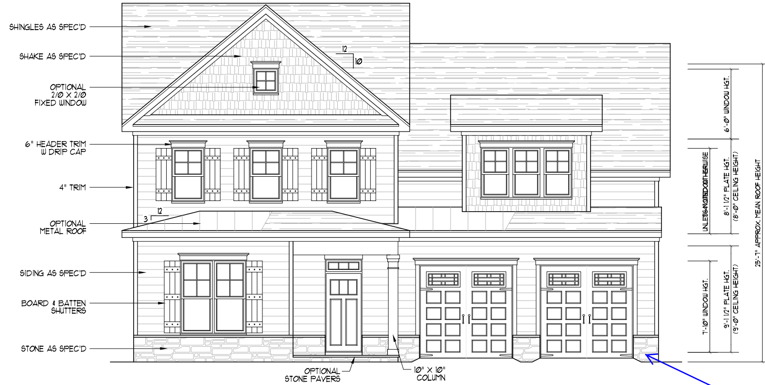
FRONT ELEVATION "B" SCALE: ----- 1/8" = 1'-0" STONE OPTION #1
