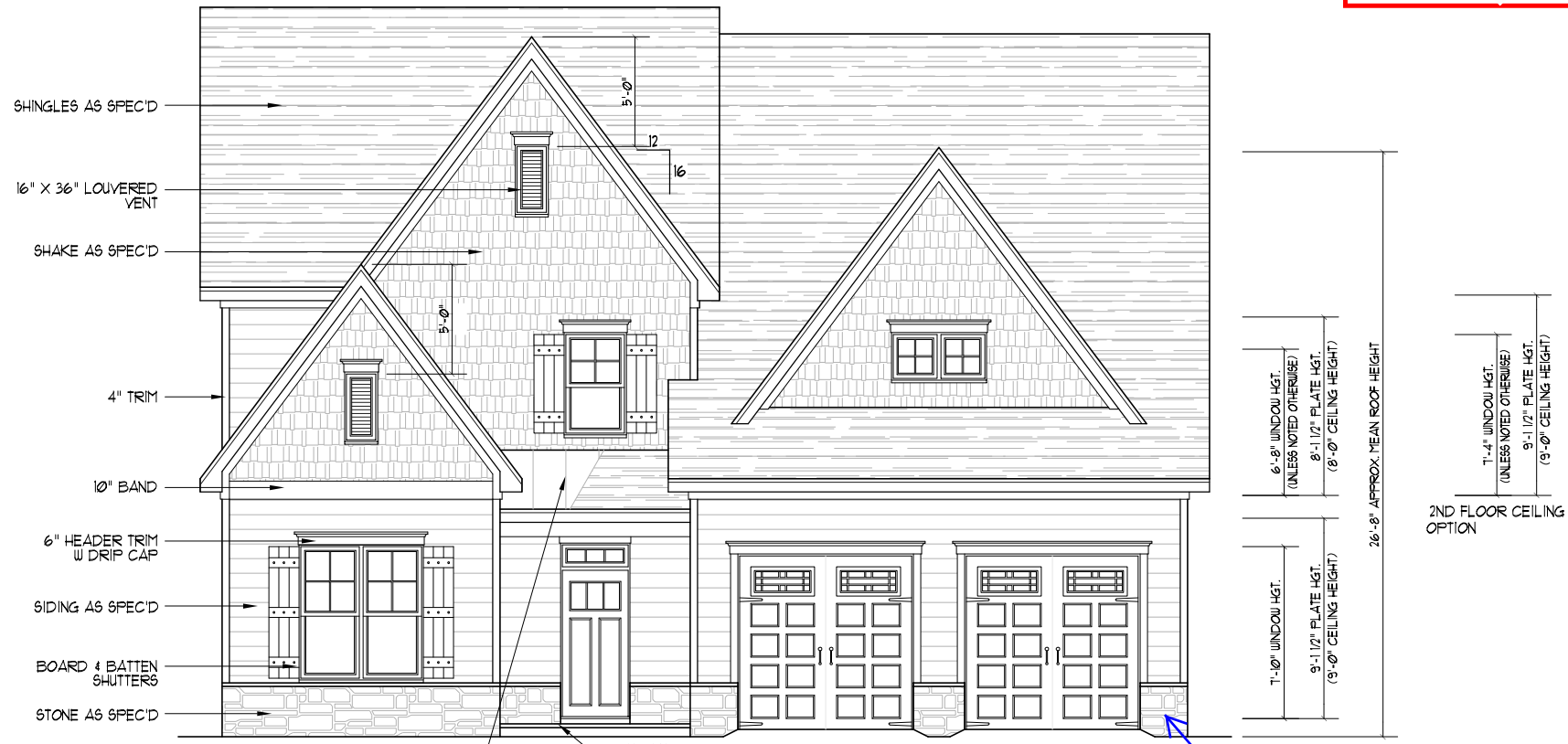
OPTIONAL METAL ROOF OPTIONAL STONE PAVING FRONT ELEVATION "B" SCALE: -----1/8" = 1'-0" STONE OPTION #1
