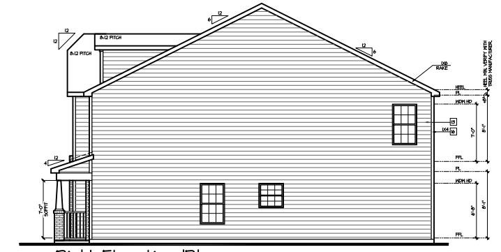
Right Elevation 'B' SCALE: 1/4"=1'-0" AT 22"x34" LAYOUT 1/8"=1'-0" AT 11"x11" LAYOUT
