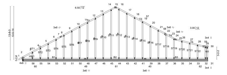
47-2-0 Plate Offsets (X,Y)-- [2:0-0-2,0-4-9], [2:0-0-1,0-0-2], [15:0-3-0,Edge], [22:0-0-0,0-1-12], [22:0-2-8,0-3-4], [23:0-2-0,0-0-0] LOADING (psf) SPACING-DEFI **PLATES** GRIP 2-0-0 CSI. I/defl I/d 20.0 TCLL (roof) Plate Grip DOL 1.15 TC 0.21 Vert(LL) -0.002-56 >999 240 MT20 244/190 Snow (Pf/Pg) 15.4/20.0
