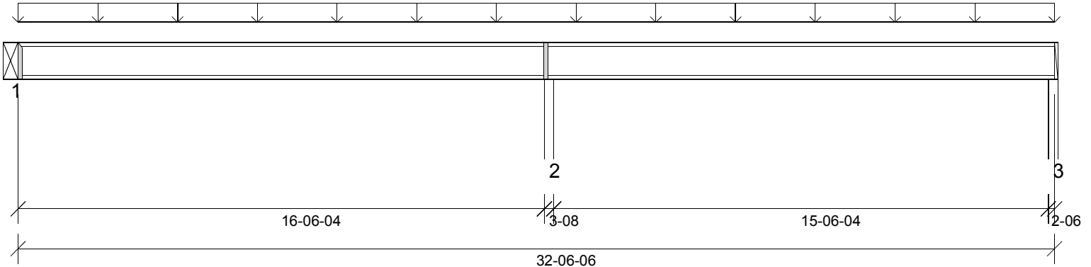
Graphical Illustration - Not To Scale Member Cut Length - 32-06-06 MemberPitch - 0/12
