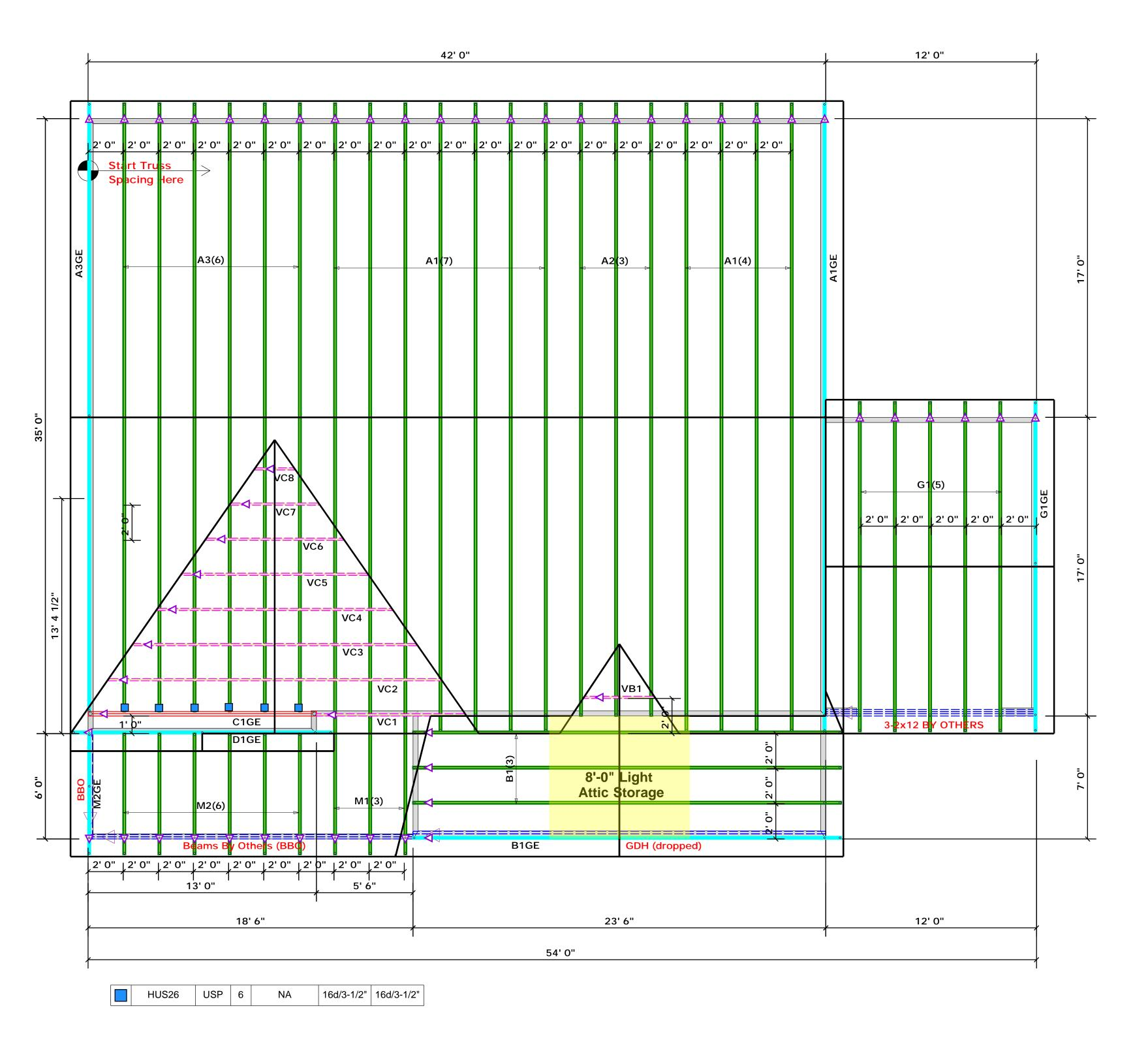
= Indicates Left End of Truss (Reference Engineered Truss Drawing) Do NOT Erect Truss Backwards
