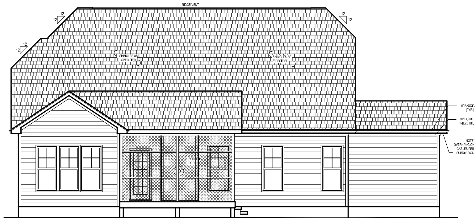
2 REAR ELEVATION - OPT. SCREEN PORCH SCALE: 1/8" = 1'-0"
