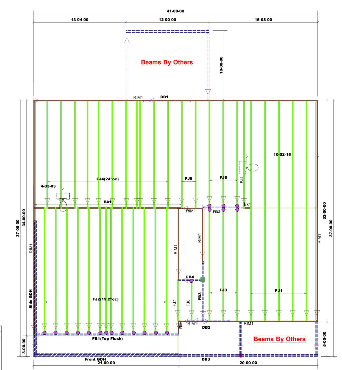
Truss Placement Plan SCALE: 1/4"=1'
