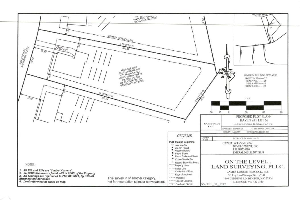
PITTMAN SOIL CONSULTING HAVEN S/D **PO BOX 1387** Owner: Address: LOT 66 **RICHLANDS, NC 28574** Location: PLACID POND DRIVE 910-330-2784 pittmansoil@yahoo.com 106 WATER INITIAL 4 BEDROOM LTAR.5 4-60' 25% REDUCTION 12-18" TB >6" SOIL COVER REQUIRED OVER SYSTEM AND 5' BEYOND SYSTEM REPAIR AREA 4 BEDROOM LTAR .5 4-60' 25% REDUCTION 12-18" TB >6" SOIL COVER REQUIRED OVER SYSTEM AND 5' BEYOND SYSTEM
