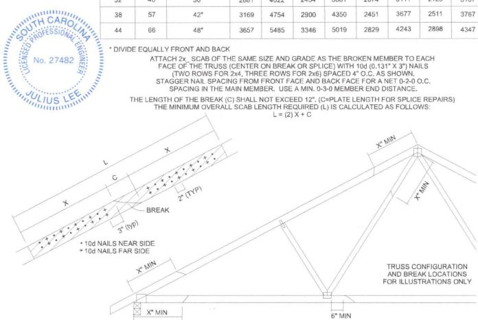
THE LOCATION OF THE BREAK MUST BE GREATER THAN OR EQUAL TO THE REQUIRED X DIMENSION FROM ANY PERIMETER BREAK OR HEEL JOINT AND A MINIMUM OF 6" FROM ANY INTERIOR JOINT (SEE SKETCH ABOVE)
