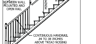
T TYPICAL DECK STAIR DETAIL SCALE 3/4" = 1'-0"
