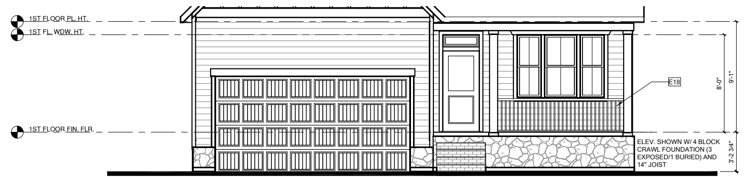
FRONT ELEVATION 'COASTAL' W/ CRAWL SPACE
