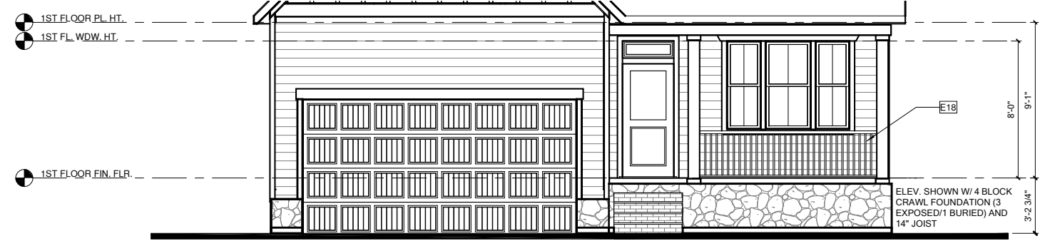
FRONT ELEVATION 'COASTAL' W/ CRAWL SPACE
