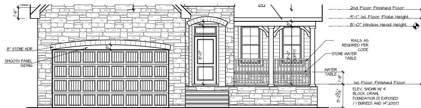
Front Elevation 'Euro' w/ Crawlspace SCALE: 1/4"=1'-0" AT 22"X34" LAYOUT 1/8"=1'-0" AT 11"X11" LAYOUT
